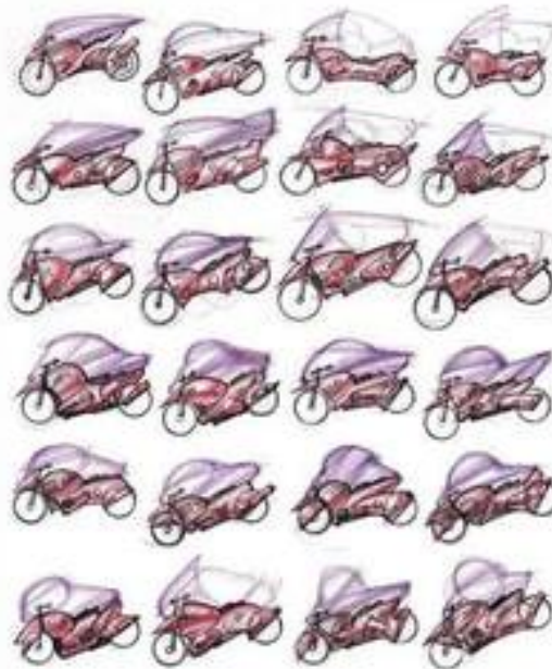
Figure VS-3B. One set of style design ideation sketches for motorcycles, completed with ball point pens.
