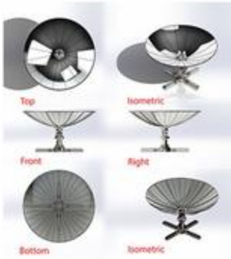
Figure 50-1. Orthographic and isometric views of the assembled Portable Solar Cooker and Oven.
