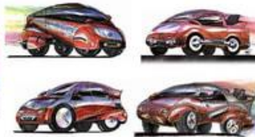
Figure VS-2A. Style design ideation and quick rendering for vans (left) and sidekicks (right), completed with fountain pens, markers, ball point pens, color pencils, and pastels.
