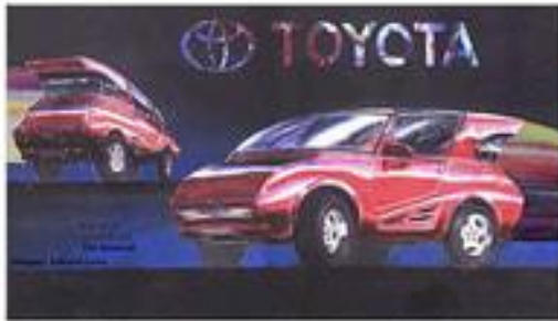
Figure VS-1C. Complete re-design and rendering of the Toyota Sidekick ("The Renewed"), completed with fountain pens, markers, ball point pens, color pencils, and pastels.
