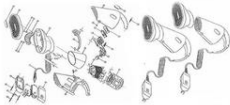
Figure HD-4B. Isometric assembly and explosion view presentation drawings for the SunSea Comfort Hair Dryer, completed manually with traditional tools and equipment such as drafting table, pencils, eraser, eraser shield, compass, ruler, triangles, T-square, French curves, circle and ellipse templates, and others.
