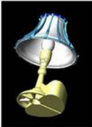
Figure TL-1. The base of the table lamp serves as a container for stationary items, such as pens, pencils, scissors, etc. (3D solid model created in AutoCAD).
