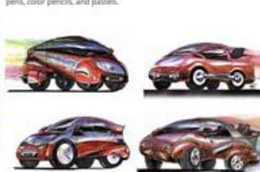
Figure V5-2A. Style design ideation and quick rendering for vans (left) and sidekicks (right), completed with fountain pens, markers, ball point pens, color pencils, and pastels.
