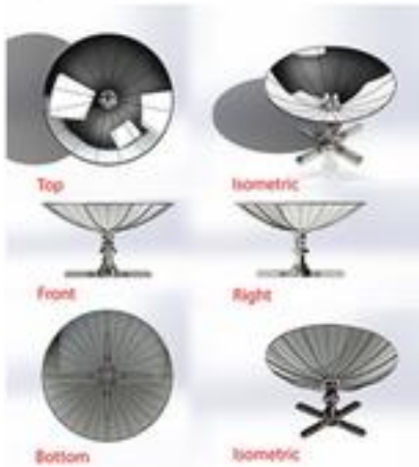
Figure SO-1. Orthographic and isometric views of the assembled Portable Solar Cooker and Oven.
