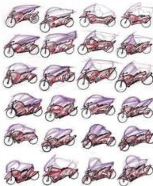
Figure V5-3B. One set of style design ideation sketches for motorcycles, completed with ball point pens.
